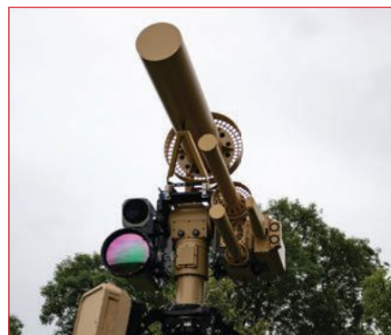
▲ Fig. 4 C-UAS system with BLACKTALON and integrated sensors.
